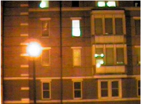
The precast concrete wall system has "excellent and uniform thermal characteristics."
